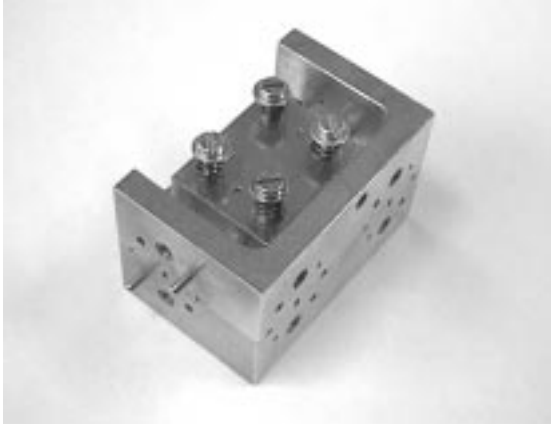
Fig. 5. Photograph of prototype filter. Port 2 (WR-8 waveguide) is seen on the left side and ports 3 and 4 on the right side.
